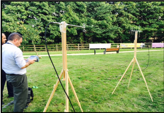
Fig. 1. Reference antenna method used to measure the LPDA gain using a calibrated biconical antenna.
