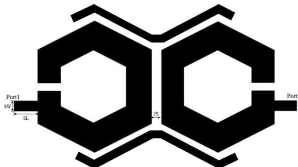
Fig1. The architecture of the proposed triple-wide band filter
