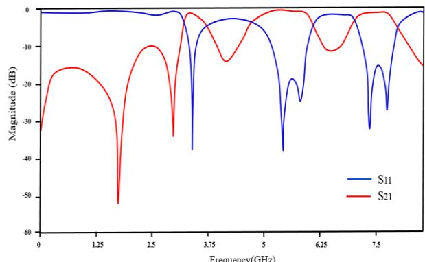
Fig2. The frequency response results of the proposed triple-band filter
